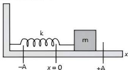
According to the figure, the linear simple harmonic oscillator consisting of a block of mass  $m$  attached to a spring. The block moves over a frictionless surface. The box, when pulled or pushed and released, executes simple harmonic motion.
