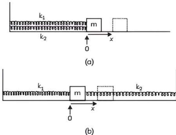
**Ans.** For figure (a), in stretching to position  $x$  from equilibrium, the restoring force to the left due to both springs is,
