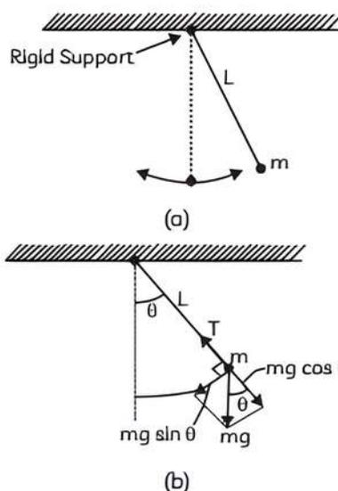
Figure (a) shows, a bob oscillating about its mean position. Figure (b) shows the radial force  $T = mg \cos\theta$  provides centripetal force but no torque about the support. The tangential force  $mg \sin\theta$  provides the restoring torque.
