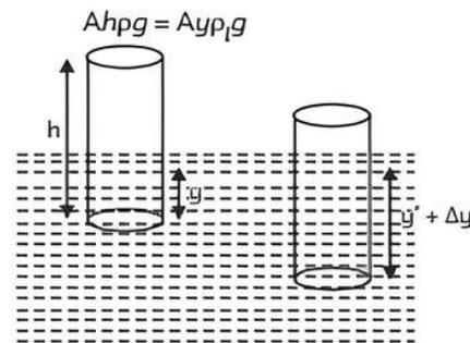
When the cylindrical cork is depressed slightly by  $\Delta y$  and released, a restoring force, equal to additional up thrust, acts on it.
